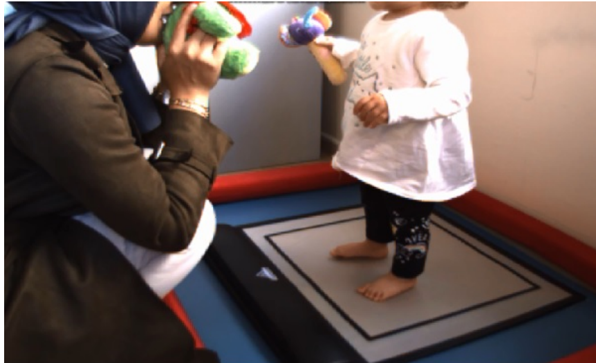
Figure 2.1: An example subject during the data collection on a pressure pad placed on top of a force plate
